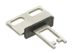
Comepi actuator tongue (key), straight mounting tab with 22mm mounting hole spacing mount, 316 stainless steel. For use with Comepi SP2K and SDM2K series safety switches.
