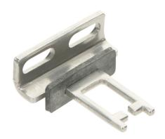
Comepi actuator tongue (key), 90 degree mounting tab with 22mm mounting hole spacing mount, 316 stainless steel. For use with Comepi SP2K and SDM2K series safety switches.
