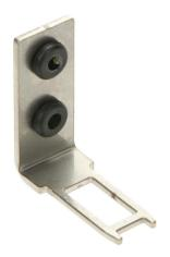
Comepi actuator tongue (key), shock absorbing, 90 degree mounting tab with 20mm mounting hole spacing mount, 316 stainless steel. For use with Comepi FEP5K series safety switches.
