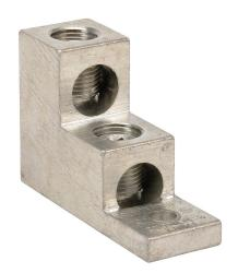
AutomationDirect box type wiring lug, line or load mount, 2 openings, #6 AWG-300 MCM wire(s). For use with GH15RT, GH15ST or GH15TT series contactors or RTD320 series overloads. Mounting hardware included.
