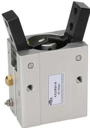
NITRA pneumatic gripper, angular, single acting, N.O., 32mm bore, 30 degrees open position, -10 degrees closed position, side mount grip, anodized aluminum body, M5 x 0.8 female ISO port(s).
