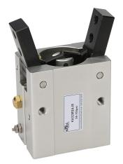
NITRA pneumatic gripper, angular, single acting, N.O., 32mm bore, 30 degrees open position, -10 degrees closed position, side mount grip, anodized aluminum body, M5 x 0.8 female ISO port(s).
