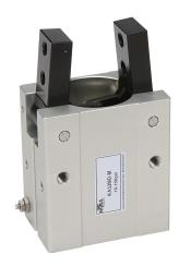
NITRA pneumatic gripper, angular, double acting, 32mm bore, 30 degrees open position, -10 degrees closed position, side mount grip, anodized aluminum body, M5 x 0.8 female ISO port(s).
