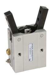
NITRA pneumatic gripper, angular, single acting, N.O., 25mm bore, 30 degrees open position, -10 degrees closed position, side mount grip, anodized aluminum body, M5 x 0.8 female ISO port(s).
