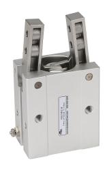
NITRA pneumatic gripper, angular, double acting, 25mm bore, 30 degrees open position, -10 degrees closed position, side mount grip, anodized aluminum body, M5 x 0.8 threaded port(s).
