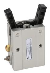
NITRA pneumatic gripper, angular, single acting, N.O., 20mm bore, 30 degrees open position, -10 degrees closed position, side mount grip, anodized aluminum body, M5 x 0.8 female ISO port(s).
