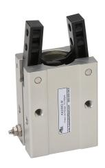
NITRA pneumatic gripper, angular, double acting, 20mm bore, 30 degrees open position, -10 degrees closed position, side mount grip, anodized aluminum body, M5 x 0.8 threaded port(s).
