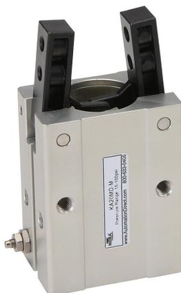
NITRA pneumatic gripper, angular, double acting, 20mm bore, 30 degrees open position, -10 degrees closed position, side mount grip, anodized aluminum body, M5 x 0.8 female ISO port(s).
