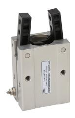
NITRA pneumatic gripper, angular, double acting, 20mm bore, 30 degrees open position, -10 degrees closed position, side mount grip, anodized aluminum body, M5 x 0.8 female ISO port(s).
