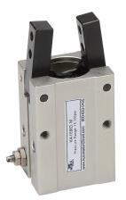
NITRA pneumatic gripper, angular, double acting, 16mm bore, 30 degrees open position, -10 degrees closed position, side mount grip, anodized aluminum body, M5 x 0.8 female ISO port(s).
