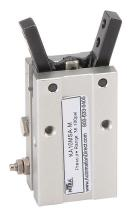
NITRA pneumatic gripper, angular, single acting, N.O., 10mm bore, 30 degrees open position, -10 degrees closed position, side mount grip, anodized aluminum body, M3 x 0.5 female ISO port(s).
