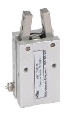
NITRA pneumatic gripper, angular, double acting, 10mm bore, 30 degrees open position, -10 degrees closed position, side mount grip, anodized aluminum body, M3 x 0.5 threaded port(s).
