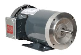
Marathon XRI premium efficiency AC induction motor, general purpose, inverter rated and 4-in-1, 3hp, 3-phase, 575 VAC, 3600rpm, TEFC, NEMA 56HC frame, rolled steel, C-face/removable rigid base mount.
