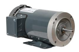
Marathon XRI premium efficiency AC induction motor, general purpose, inverter rated and 4-in-1, 2hp, 3-phase, 575 VAC, 1800rpm, TEFC, 56HC frame, rolled steel, C-face/removable rigid base mount.
