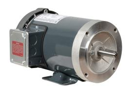
Marathon XRI premium efficiency AC induction motor, general purpose, inverter rated and 4-in-1, 1-1/2hp, 3-phase, 575 VAC, 3600rpm, TEFC, NEMA 56C frame, rolled steel, C-face/removable rigid base mount.
