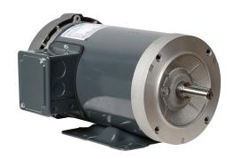
Marathon XRI premium efficiency AC induction motor, general purpose, inverter rated and 4-in-1, 1hp, 3-phase, 575 VAC, 1800rpm, TEFC, 56HC frame, rolled steel, C-face/removable rigid base mount.
