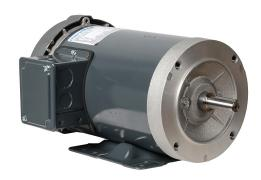
Marathon XRI premium efficiency AC induction motor, general purpose, inverter rated and 4-in-1, 1hp, 3-phase, 575 VAC, 1800rpm, TEFC, NEMA 56HC frame, rolled steel, C-face/removable rigid base mount.
