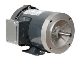
Marathon XRI standard efficiency AC induction motor, general purpose, inverter rated and 4-in-1, 3/4hp, 3-phase, 575 VAC, 1800rpm, TEFC, NEMA 56C frame, rolled steel, C-face/removable rigid base mount.
