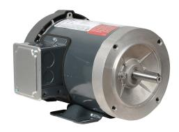
Marathon XRI standard efficiency AC induction motor, general purpose, inverter rated and 4-in-1, 1/2hp, 3-phase, 575 VAC, 1800rpm, TEFC, NEMA 56C frame, rolled steel, C-face/removable rigid base mount.
