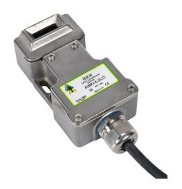
IDEM safety switch, tongue (key) interlock, hazardous location rated, 180-degree adjustable head, (2) N.C. safety output(s), (2) N.O. monitoring output(s), 58 x 104 x 37mm, 316 stainless steel body, 316 stainless steel head.
