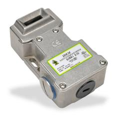
IDEM safety switch, tongue (key) interlock, 180-degree adjustable head, (2) N.C. safety output(s), (2) N.O. monitoring output(s), 58 x 104 x 37mm, 316 stainless steel body, 316 stainless steel head.
