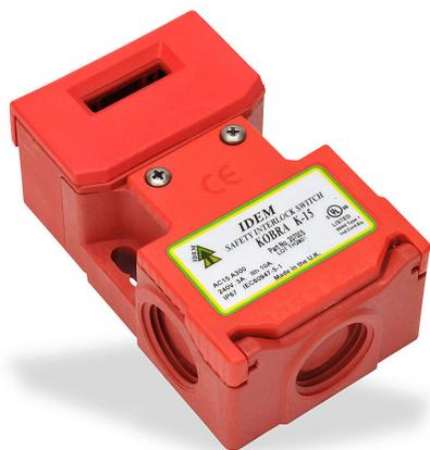
IDEM safety switch, tongue (key) interlock, 180-degree adjustable head, (3) N.C. safety output(s), 54 x 88 x 34mm, plastic body, plastic head.
