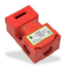
IDEM safety switch, tongue (key) interlock, 180-degree adjustable head, (2) N.C. safety output(s), (1) N.O. monitoring output(s),  $54 \times 34$ mm, plastic body, plastic head.
