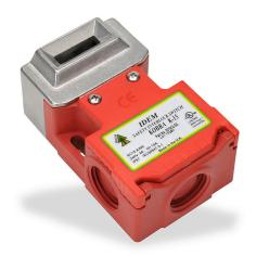
IDEM safety switch, tongue (key) interlock, 180-degree adjustable head, (2) N.C. safety output(s), (1) N.O. monitoring output(s),  $54 \times 91 \times 37$ mm, plastic body, 316 stainless steel head.
