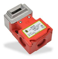
IDEM safety switch, tongue (key) interlock, 180-degree adjustable head, (2) N.C. safety output(s), (1) N.O. monitoring output(s), 54 x 91 x 37mm, plastic body, 316 stainless steel head.
