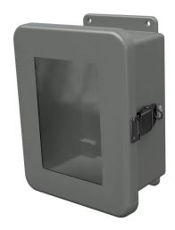
Stahlin JW series enclosure, NEMA 1/3R/4X/6P/12, 8 x 6 x 4in (HxWxD), wall mount, fiberglass reinforced polyester, gray, single-door, (1) quick-release latch, padlock hasp and staple, SAR acrylic window.
