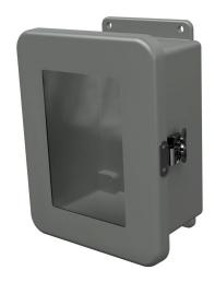
Stahlin JW series enclosure, NEMA 1/3R/4X/6P/12, 8 x 6 x 4in (HxWxD), wall mount, fiberglass reinforced polyester, gray, single-door, (1) twist-lock latch, SAR acrylic window.
