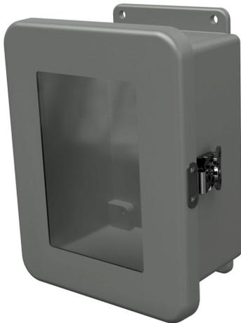
Stahlin JW series enclosure, NEMA 1/3R/4X/6P/12, 8 x 6 x 4in (HxWxD), wall mount, fiberglass reinforced polyester, gray, single-door, (1) twist-lock latch, SAR acrylic window.
