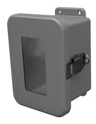
Stahlin JW series enclosure, NEMA 1/3R/4X/6P/12, 6 x 4 x 4in (HxWxD), wall mount, fiberglass reinforced polyester, gray, single-door, (1) quick-release latch, padlock hasp and staple, SAR acrylic window.
