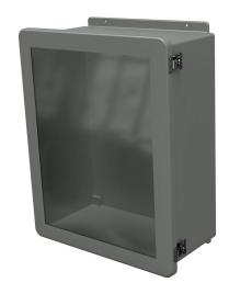
Stahlin JW series enclosure, NEMA 1/3R/4X/6P/12, 20 x 16 x 8in (HxWxD), wall mount, fiberglass reinforced polyester, gray, singledoor, (2) twist-lock latches, SAR acrylic window.
