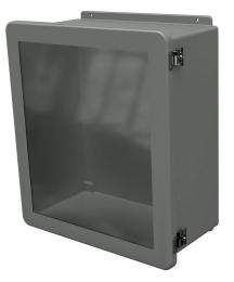
Stahlin JW series enclosure, NEMA 1/3R/4X/6P/12, 18 x 16 x 8in (HxWxD), wall mount, fiberglass reinforced polyester, gray, single-door, (2) twist-lock latches, SAR acrylic window.
