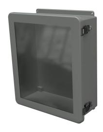
Stahlin JW series enclosure, NEMA 1/3R/4X/6P/12,  $16 \times 14 \times 6$ in (HxWxD), wall mount, fiberglass reinforced polyester, gray, singledoor, (2) quick-release latches, padlock hasp and staple, SAR acrylic window.
