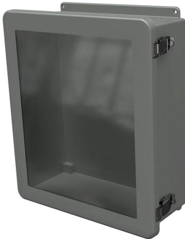
Stahlin JW series enclosure, NEMA 1/3R/4X/6P/12, 16 x 14 x 6in (HxWxD), wall mount, fiberglass reinforced polyester, gray, single-door, (2) quick-release latches, padlock hasp and staple, SAR acrylic window.
