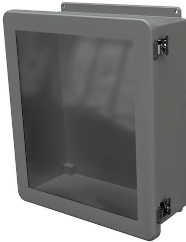
Stahlin JW series enclosure, NEMA 1/3R/4X/6P/12, 16 x 14 x 6in (HxWxD), wall mount, fiberglass reinforced polyester, gray, single-door, (2) twist-lock latches, SAR acrylic window.
