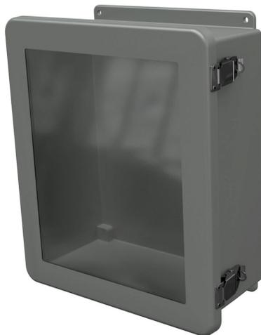
Stahlin JW series enclosure, NEMA 1/3R/4X/6P/12, 14 x 12 x 6in (HxWxD), wall mount, fiberglass reinforced polyester, gray, single-door, (2) quick-release latches, padlock hasp and staple, SAR acrylic window.
