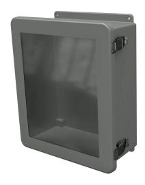
Stahlin JW series enclosure, NEMA 1/3R/4X/6P/12,  $14 \times 12 \times 6$ in (HxWxD), wall mount, fiberglass reinforced polyester, gray, singledoor, (2) quick-release latches, padlock hasp and staple, SAR acrylic window.
