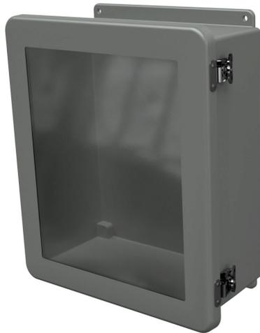
Stahlin JW series enclosure, NEMA 1/3R/4X/6P/12, 14 x 12 x 6in (HxWxD), wall mount, fiberglass reinforced polyester, gray, single-door, (2) twist-lock latches, SAR acrylic window.
