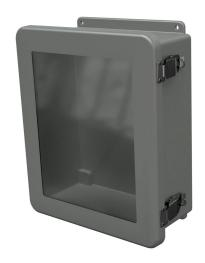
Stahlin JW series enclosure, NEMA 1/3R/4X/6P/12,  $12 \times 10 \times 5$ in (HxWxD), wall mount, fiberglass reinforced polyester, gray, singledoor, (2) quick-release latches, padlock hasp and staple, SAR acrylic window.
