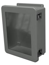
Stahlin JW series enclosure, NEMA 1/3R/4X/6P/12, 12 x 10 x 5in (HxWxD), wall mount, fiberglass reinforced polyester, gray, single-door, (2) twist-lock latches, SAR acrylic window.
