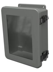
Stahlin JW series enclosure, NEMA 1/3R/4X/6P/12, 10 x 8 x 4in (HxWxD), wall mount, fiberglass reinforced polyester, gray, singledoor, (2) quick-release latches, padlock hasp and staple, SAR acrylic window.
