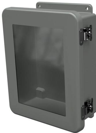
Stahlin JW series enclosure, NEMA 1/3R/4X/6P/12, 10 x 8 x 4in (HxWxD), wall mount, fiberglass reinforced polyester, gray, single-door, (2) twist-lock latches, SAR acrylic window.
