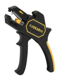
JOKARI automatic cutting and stripping tool, compatible with round wire, non-slip pistol grip, special steel hardened cutting edges, self-adjusting, 24-10 AWG wire stripping capacity, 14 AWG cutting capacity.
