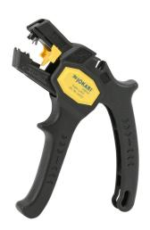
JOKARI automatic cutting and stripping tool, compatible with round wire, pistol grip, special steel hardened cutting edges, self-adjusting, 24-10 AWG wire stripping capacity, 14 AWG cutting capacity.
