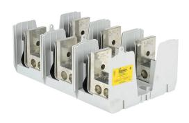
Bussmann modular fuse block, accepts J fuses, 600A, 600V, 3-pole, 2 line/2 load opening(s) per pole, (2) 4 AWG-500 MCM copper or aluminum, box lug, panel mount.
