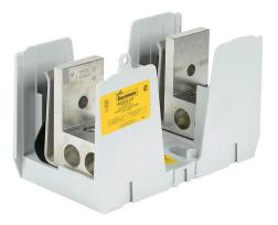
Bussmann modular fuse block, accepts J fuses, 600A, 600V, 1-pole, 2 line/2 load opening(s) per pole, (2) 4 AWG-500 MCM copper or aluminum, box lug, panel mount.
