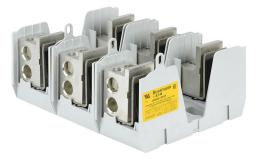
Bussmann modular power distribution fuse block, multi-wire, accepts J fuses, 400A, 600V, 3-pole, 2 line/6 load opening(s) per pole, box lug, panel mount.
