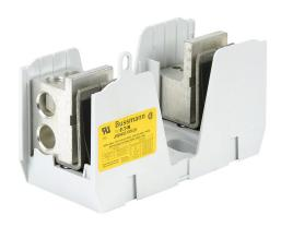
Bussmann modular power distribution fuse block, multi-wire, accepts J fuses, 400A, 600V, 1-pole, 2 line/6 load opening(s) per pole, box lug, panel mount.
