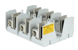
Bussmann modular power distribution fuse block, multi-wire, accepts J fuses, 400A, 600V, 3-pole, 1 line/6 load opening(s) per pole, box lug, panel mount.
