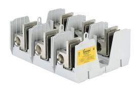
Bussmann modular fuse block, accepts J fuses, 400A, 600V, 3-pole, 4 AWG-600 MCM copper or aluminum, box lug, panel mount.
