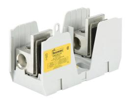
Bussmann modular fuse block, accepts J fuses, 400A, 600V, 1-pole, 4 AWG-600 MCM copper or aluminum, box lug, panel mount.
