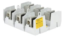
Bussmann modular power distribution fuse block, multi-wire, accepts J fuses, 200A, 600V, 3-pole, 1 line/6 load opening(s) per pole, box lug, panel mount.
