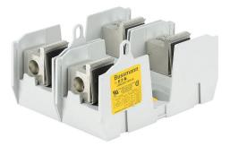
Bussmann modular power distribution fuse block, multi-wire, accepts J fuses, 200A, 600V, 2-pole, 1 line/6 load opening(s) per pole, box lug, panel mount.
