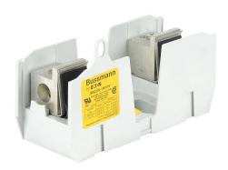
Bussmann modular power distribution fuse block, multi-wire, accepts J fuses, 200A, 600V, 1-pole, 1 line/6 load opening(s) per pole, box lug, panel mount.
