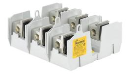
Bussmann modular fuse block, accepts J fuses, 200A, 600V, 3-pole, 6 AWG-250 MCM copper or aluminum, box lug, panel mount.
