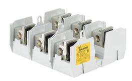
Bussmann modular fuse block, accepts J fuses, 200A, 600V, 3-pole, 6 AWG-250 MCM copper or aluminum, box lug, panel mount
